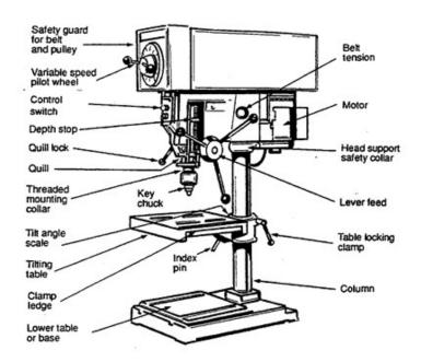
Diagram of a Typical Drill Press
